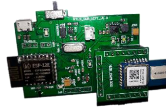
Fig. 8. Developed RTLS board.
