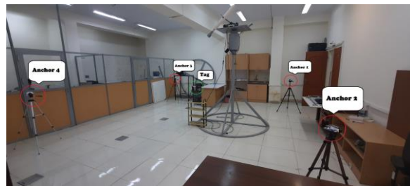
Fig. 10. NLOS condition positioning environment.
